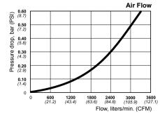
Flow capacity is measured at 6 bar (87 PSI) inlet pressure, and pressure drop at 0.5 bar (7 PSI). Thread connections are listed according to ISO Standards (see Page 82 for more information) Check with an authorized CEJN distributor for availability and prices.
